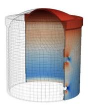
Illustration of coupled heat and moisture analysis and long-term mechanical analysis of concrete pressure vessel.
