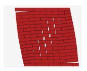
Illustration of failure analysis of masonry wall using standard 2D elements combined with interface elements and elastoplastic constitutive law to model nonlinear mortar behavior.
