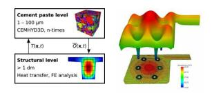
Hydrating concrete produces a significant amount of hydration heat, causing several problems in massive elements. The multiscale simulation helped to find an optimal position of cooling pipes and cooling regime on an arch of Opárno bridge, Czech Republic.
