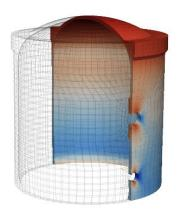
Illustration of coupled heat and moisture analysis and long-term mechanical analysis of concrete pressure vessel.
