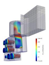
Illustration of nonlinear analysis of a hinge holding hermetic door in an atomic power plant. The model with J2 plasticity without hardening helped evaluating the amount of dissipated energy in the case of a vapour explosion.
